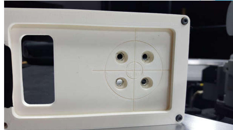
3d printed sample holder with visual target
