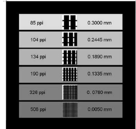
A good **estimation of the MTF (CTF)** of the imaging system is obtained with two targets.
