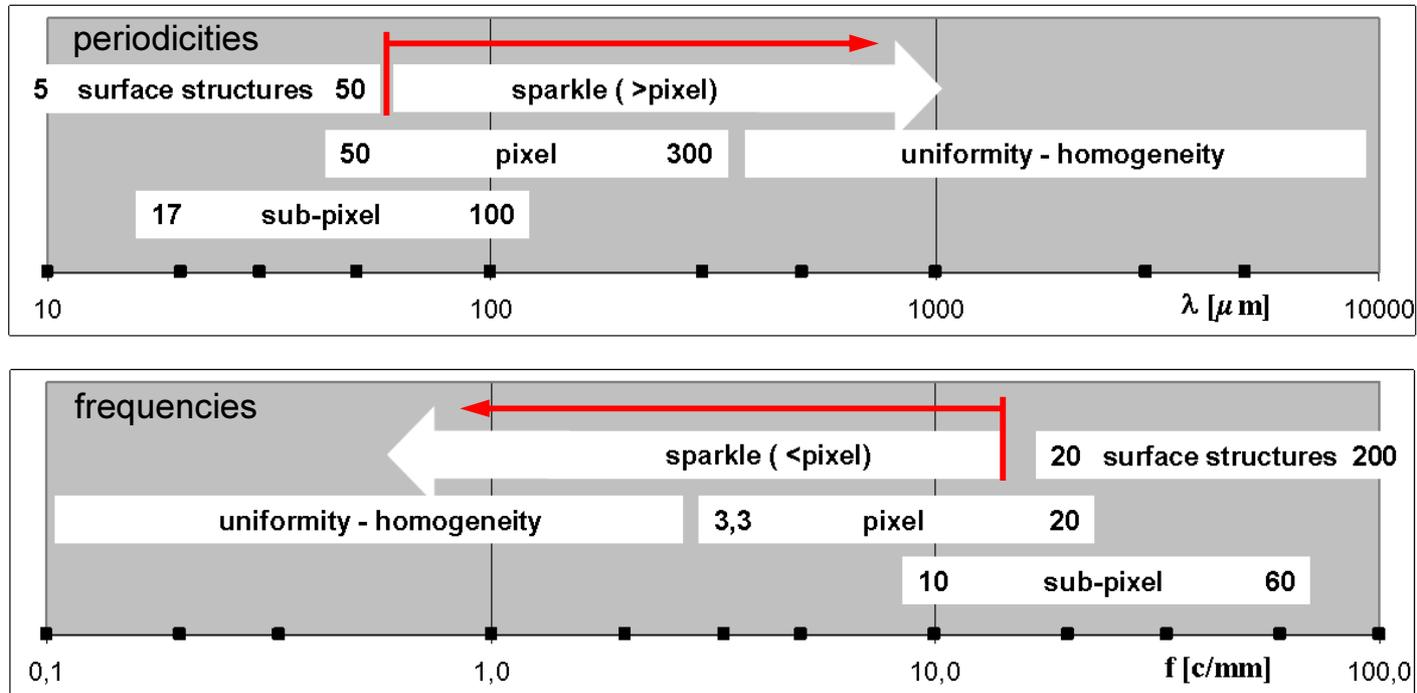
The display pixel matrix introduces **periodic intensity variations** while visual sparkle is caused by **statistic intensity modulations** (vs. location on the display and vs. direction of observation).
