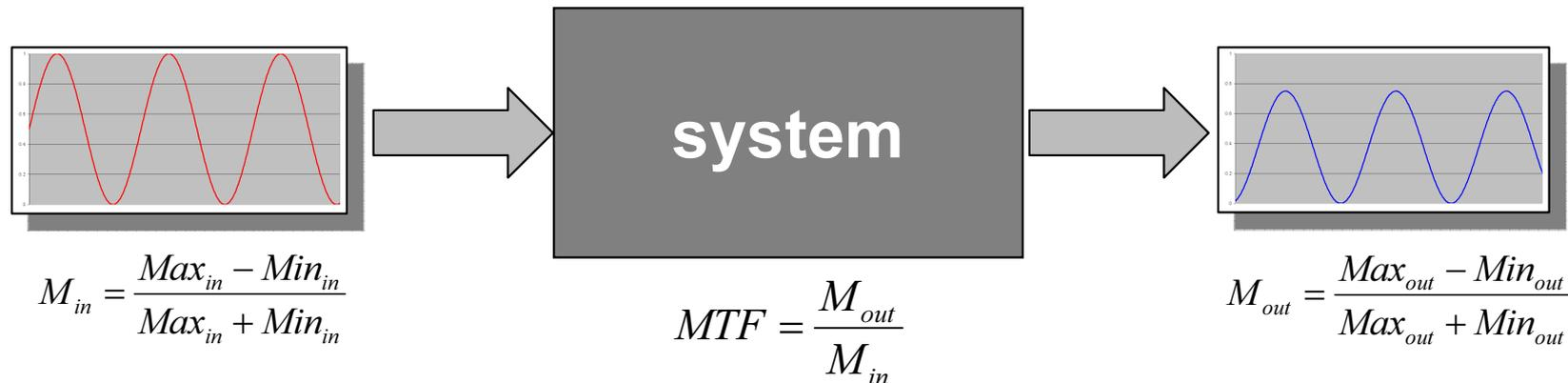
In an electronic imaging system the MTF of the system is given by the MTF of the optics and the MTF of the detector array.
