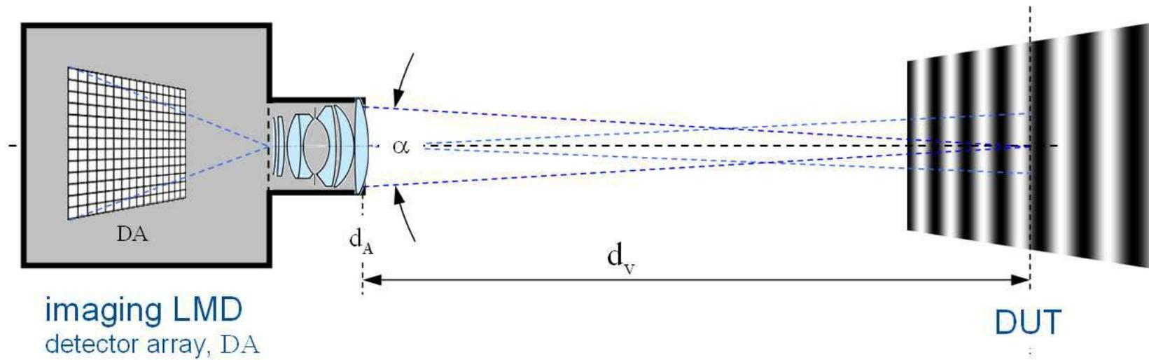
If a continuous light intensity distribution,  $L(x, y)$ , of the DUT contains no spatial frequencies higher than  $B$  (cycles / distance  $x, y$ ), the distribution is completely specified by sampling it with a series of pulses placed  $1/(2 \cdot B)$  apart in both  $x$  and  $y$  direction.
