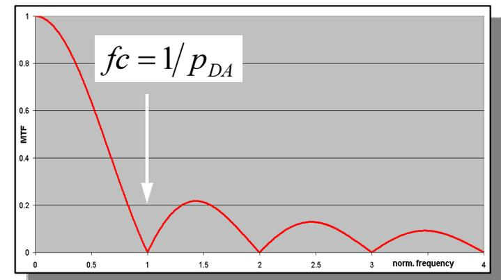
The cutoff frequency of the MTF of the detector array (first zero),  $f_c$ , is given by the pitch of its elements,  $p_{DA}$ .
