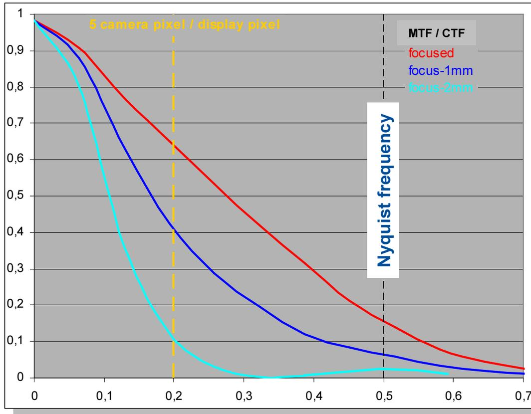
Effect of de-focus on the MTF / CTF of an electronic imaging system with  $f = 50$  mm,  $F\#5.6$ , at a working distance of 200 mm.
